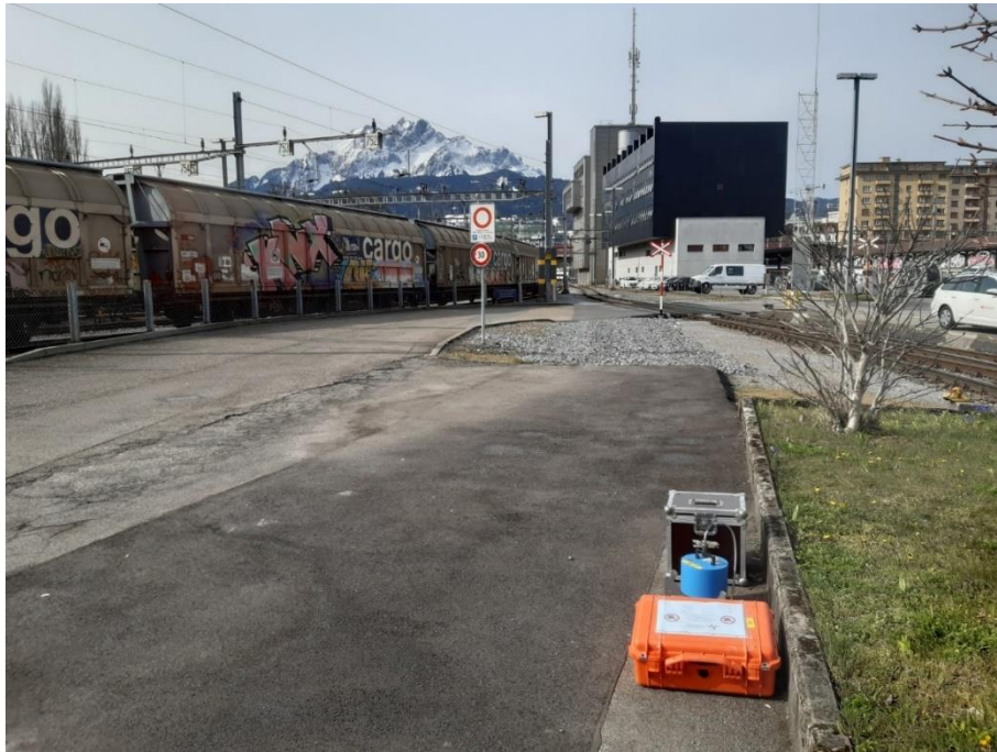
Figure 16. Example of measurement of ambient noise close to the Lucerne train station during the survey in April 2021. The setup consists of a Lennartz 5-s sensor and Centaur digitizer. Photo: Paulina Janusz
