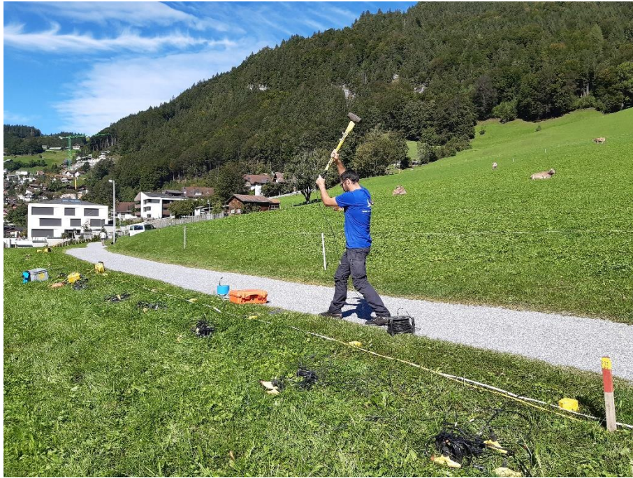
Figure 7. MASW using hammer source during site characterization of seismic station belonging to Swiss Strong Motion Network (SSMNet) (Hobiger et al., 2021; Michel et al., 2014). Photo: Paulina Janusz
